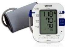
This sensor is a blood pressure monitor that could transfer data using Bluetooth technology and it is certified by the Continua Alliance and implements the 11073 communication protocol.
