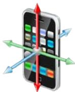
The Physical Activity Detector (PAD) is an android based mobile service which uses the internal accelerometer of a smartphone to detect the type of activity that the user is performing: resting, waking or running. This sensor is available for both clinical domains.
