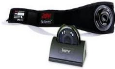
The Zephyr ECG belt allows monitoring the patient hearth rhythm/heart rate (dual mode) and communicates with the smartphone via Bluetooth. This device is already CE approved for use. The sensor includes a single-lead ECG monitor, an accelerometer to detect the level of physical activity and a respiration monitor for AF patients.
